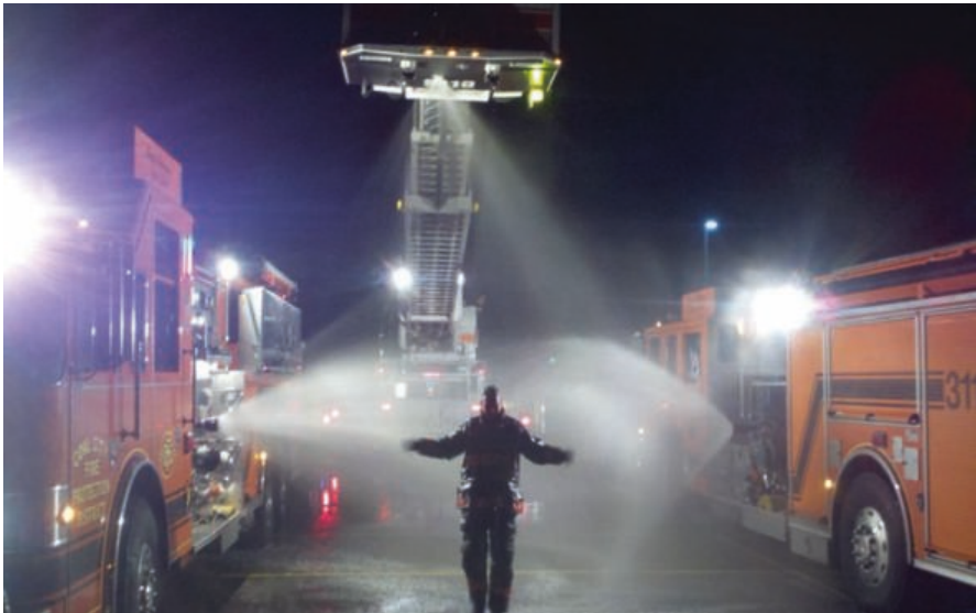
Fig. 9.1 Ladder pipe system (Fire Department Mass Decon [Internet] 2011)
